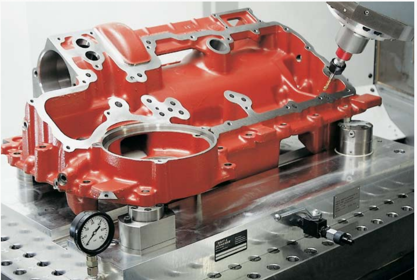
Workpiece clamping device, equipped with hydraulic pull-down clamps, version „centric“ at front left, and „eccentric“ at right.
