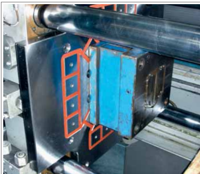
Magnetic clamping plate with an injection mould
