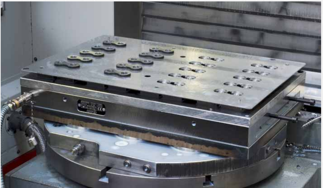
Rapid and economical clamping of asymmetrical components; shaped carrier plate in use with individual components: An additional thin sheet metal plate is fixed on the shaped carrier plate. Support on four poles guarantees the fit in the axes, and an optimal magnetic force results.
