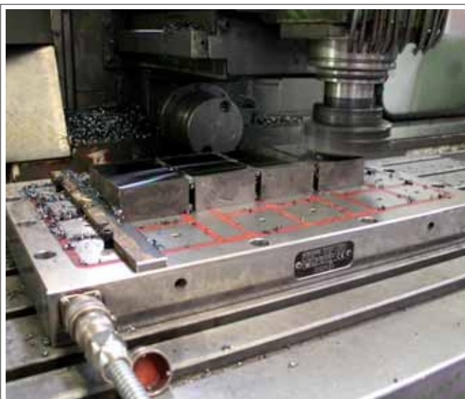
The workpieces were positioned directly on the magnetic clamping plate and milled. A stop strip and intermediate bars further facilitate an optimum clamping on the magnetic clamping plate.
