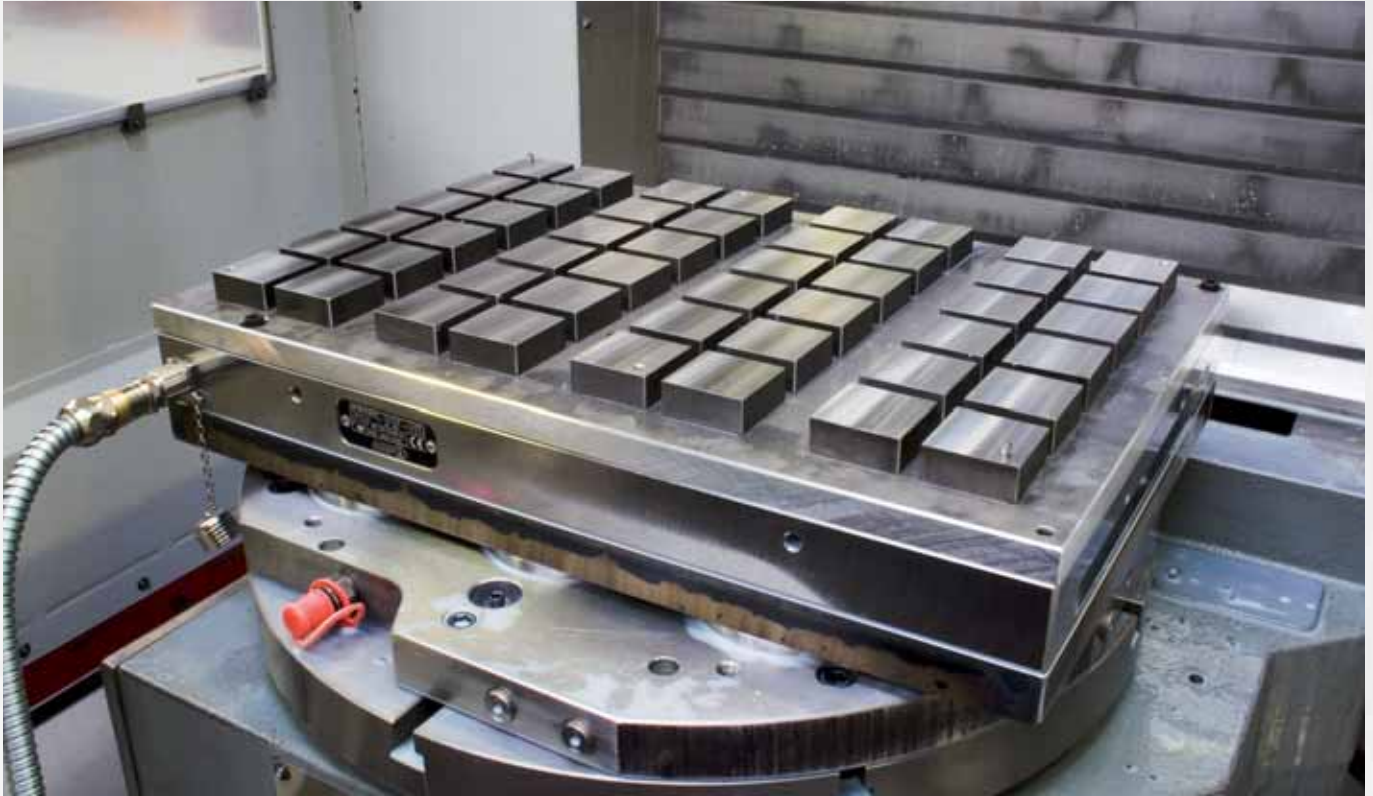
Shaped carrier plate as base plate. With this plate, you can machine individual small or asymmetrical parts that cannot be clamped other than on a magnetic clamping plate.
