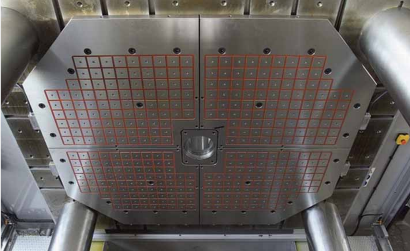
Four individual magnetic clamping plates are bolted into an injection moulding machine and connected to one another.
