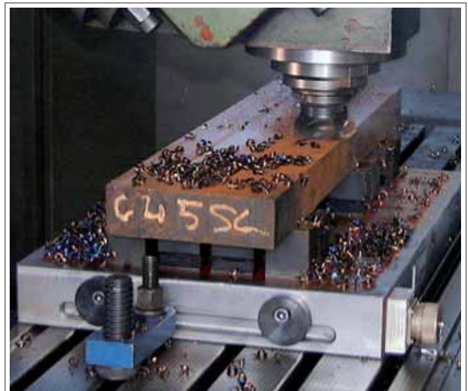
Flame-cut workpiece is clamped on fixed and movable pole extensions and milled. The discharge cable is unplugged during the machining.
