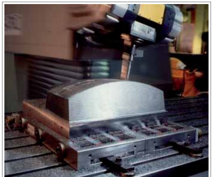
The workpiece for the mould is directly positioned on two magnetic clamping plates and all 5 sides are milled with one clamping.
