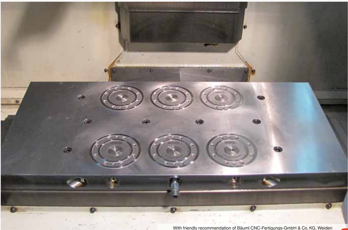
The Zero-Point System used together with the AMF magnetic clamping technology With friendly recommendation of Bäuml CNC-Fertigungs-GmbH & Co. KG, Weiden
