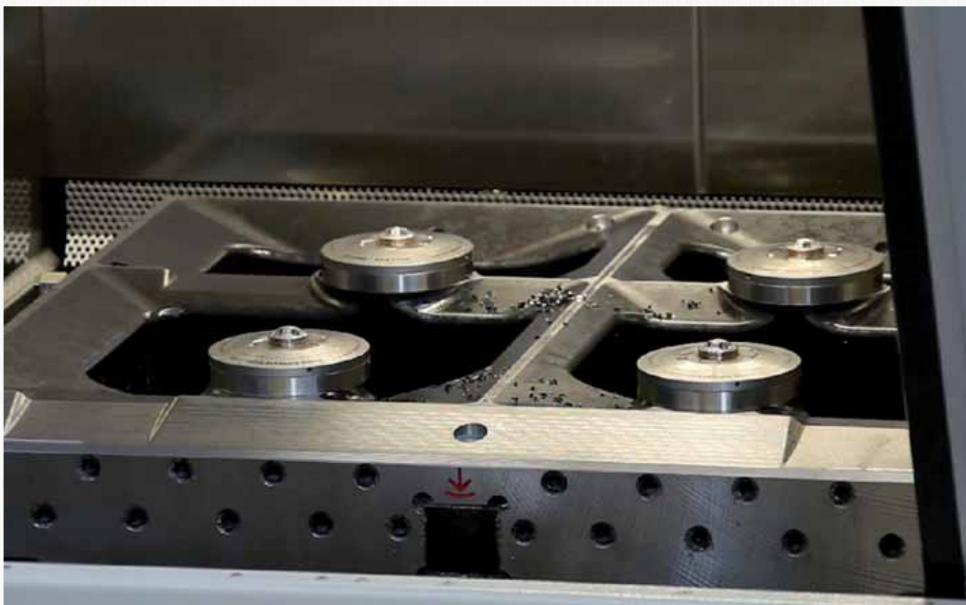
„Turbine“ high-end clamping module (order no. 420919) in use in a fully automated production process with robot loading.
