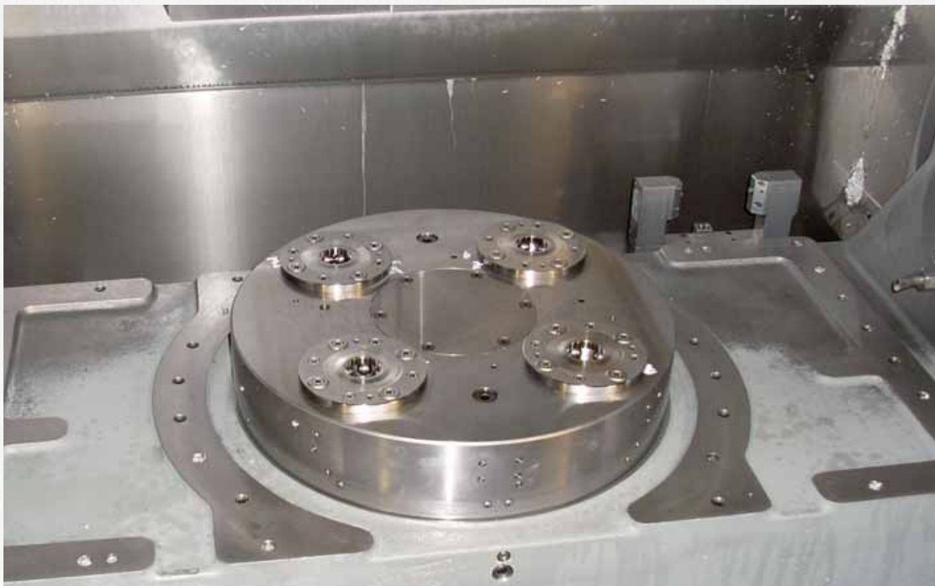
Automation solution (order no. 427161) with lock and support control as well as nipple sensing in use in a fully automated production process with robot loading.
