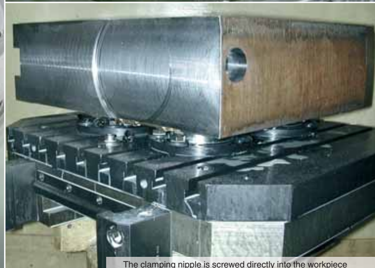
The clamping nipple is screwed directly into the workpiece
