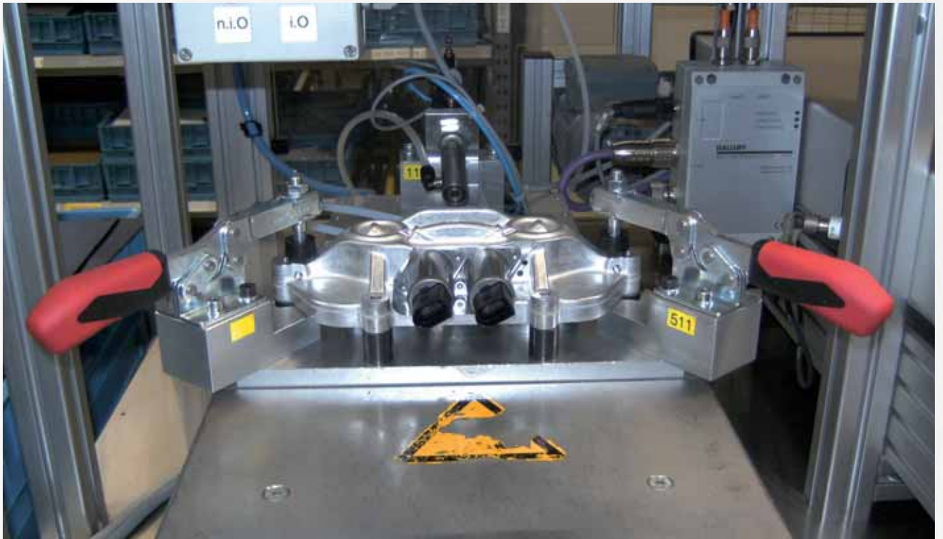
Horizontal toggle clamp no. 6830 in application on a fixture for leak testing. In this case a component to the camshaft adjustment is mounted.
