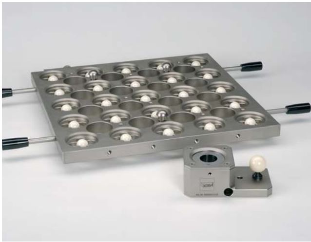
Fig. 1: KOBA-check sphere plate in horizontal construction with insulating handles and probe test unit
